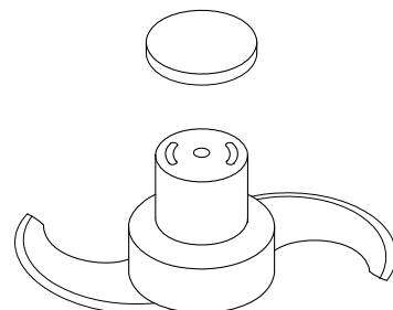
There is a removable cap attached to the top of the S-blade assembly. This cap should be removed when cleaning the blade assembly.
