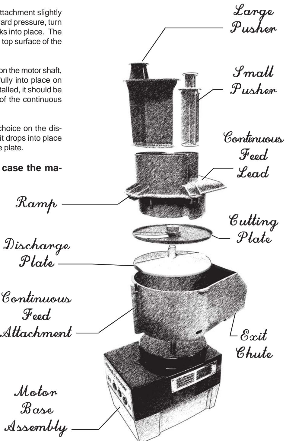
The continuous feed lead, with the pushers in place, provides protection from the cutting disc. When the lead is turned to its closed position with the ramp in place over the pin, a safety switch is activated, and the machine can be turned on and off by use of the push buttons. If the lead is not in the closed position, the buttons will not function.
