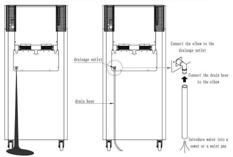
In case of water overflow from the re-evaporation tray on the back of an upright cabinet the user must connect a drain hose (Inner diameter 10 mm) to the tray. The hose shall lead to a sewer or a water pan. The user can connect the drainage outlet and the drain hose using the elbow in the accessories. The user need to prepare a 10mm inner diameter drainage hose, which is not included in the accessories.
