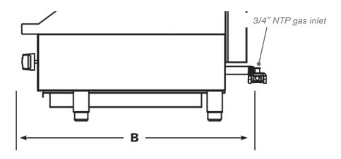
CLEARANCES These units can be installed on non-combustible countertops using the provided 3.5 inch (88.9 mm) legs or on a combustible floor using a minimum 28.5-inch (723.9 mm) tall stand. The back and both sides must be at least six inches (152.4 mm) from any combustible surface.
