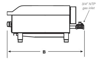
CLEARANCES These units can be installed on non-combustible countertops using the provided 3.5 inch (88.9 mm) legs or on a combustible floor using a minimum 28.5-inch (723.9 mm) tall stand. The back and both sides must be at least six inches (152.4 mm) from any combustible surface.
